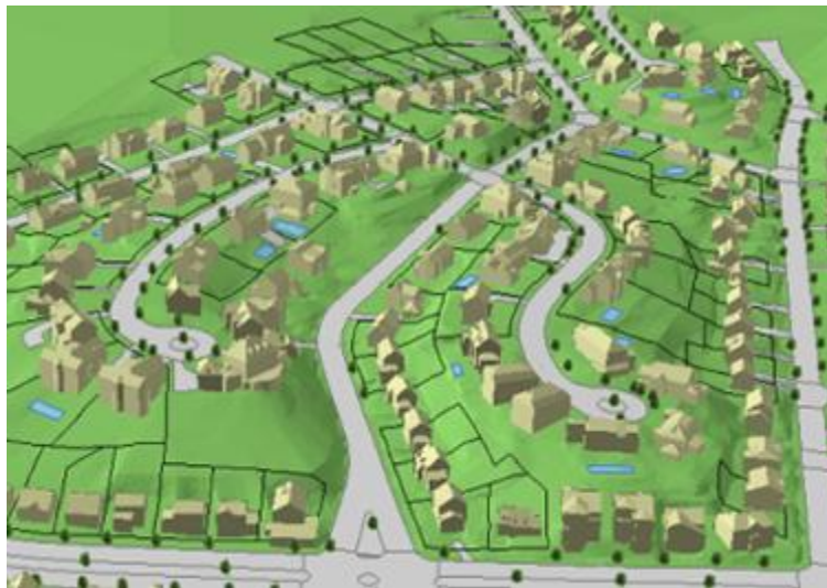
Figure 6: 3D Scenes with draped 2D features which take on the z-coordinates of the DTM
